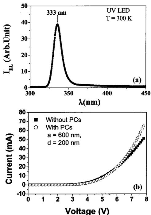
FIG. 3. (a) Typical EL spectrum of the 333 nm UV LEDs. (b) The I-V characteristics of UV LEDs with PCs ( $a = 600\ \text{nm}$ ,  $d = 200\ \text{nm}$ ) and without PCs.
